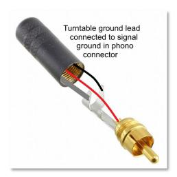
Some turntables have a thin "ground" wire alongside the phono cables. This wire normally connects to the metal components of the tonearm and to the plate which carries the main turntable bearing.
